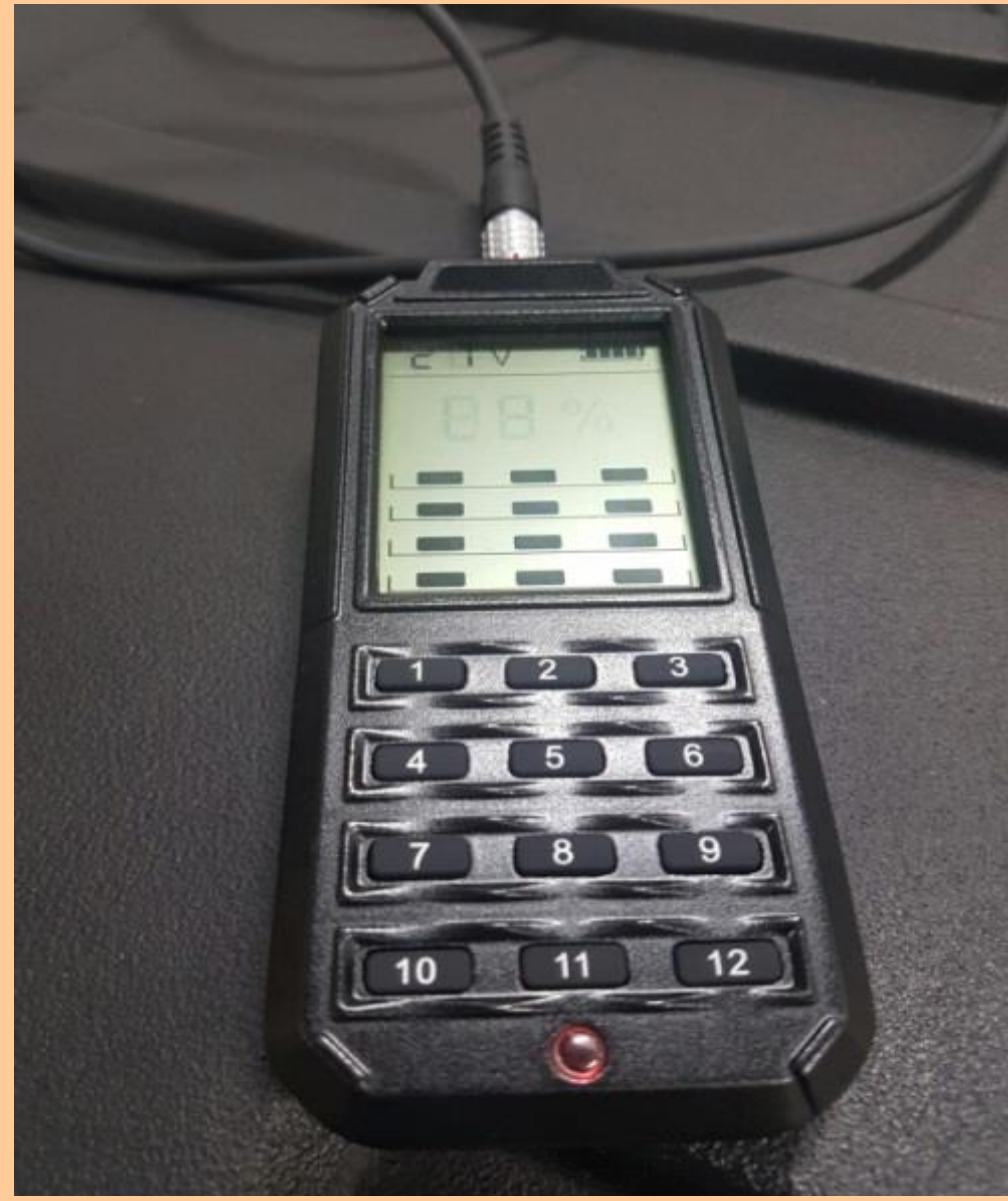
Simple Control Panel for remote operation
